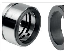
Characteristics:Single seal multiple springsDouble DirectionalBalancedAccording to DIN 24960Limit of applications:Pressurep = 25 barSpeedv = 20 m/sTemperaturet = -20 + 200°CAvailable:stationary seats type OL/CC or CL
