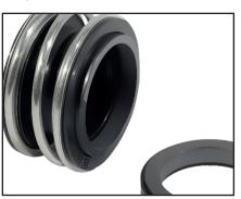
Characteristics:Single Mechanical SealRubber Bellows sealDouble DirectionalUnbalancedLimit of applications:Pressurep = 12 barSpeedv = 10 m/sTemperature $t = -30 + 200^{\circ}$ CAvailable:FG1-FG2-FG3 (metric/inch)
