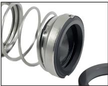
Characteristics:Single Mechanical SealRubber Bellows sealDouble DirectionalUnbalanced - According to DIN 24960Limit of applications:Pressurep = 12 barSpeedv = 15 m/sTemperature $t = -30 + 200^{\circ}C$ Available: FP/S-FP/T3S
